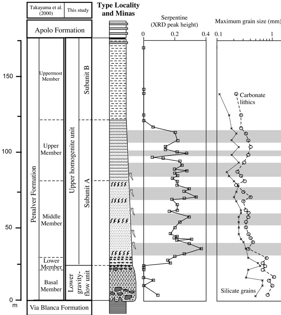
**Figure 7.** Slight vertical variations in mineral composition and grain size in the upper homogenite unit of the Peñaalver Formation at the type locality.
