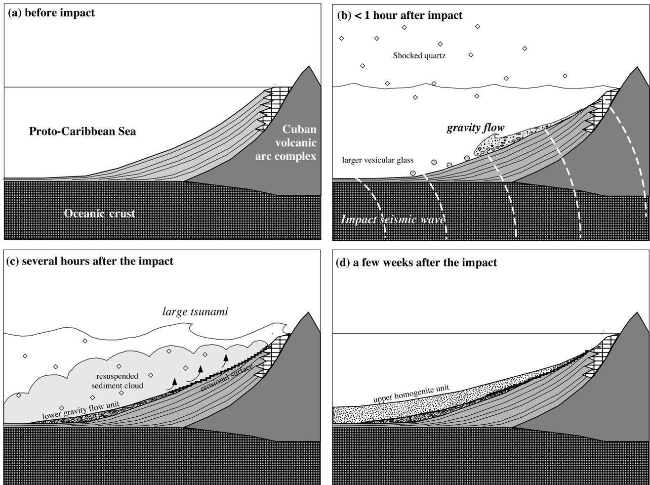
**Figure 12.** A cartoon showing the depositional processes of the deep-sea K/T boundary deposit (the Peñalver Formation as an example). (a) The situation immediately before the impact. (b) The impact seismic wave triggered the gravity flow. (c) Large tsunami waves associated with the impact eroded the deep sea floor and formed a resuspended sediment cloud. (d) Resuspended sediment particles settled down to form homogenite.
