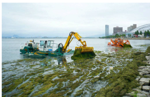
Removal operations by a specialized water-plant harvester boat in southern Otsu City. (Source: Lake Biwa Policy Division, Shiga Prefectural Government.)
