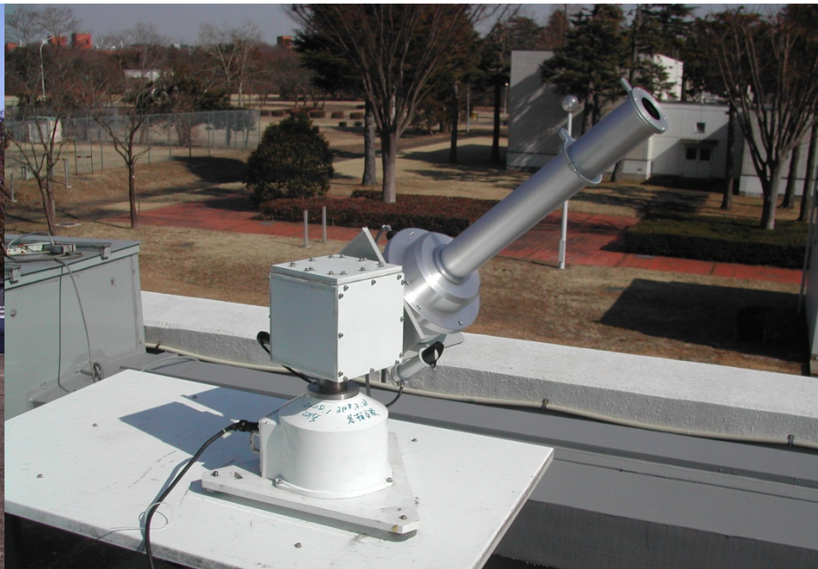
Use of collimation tube
