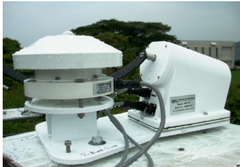
Type: MS-700 with shadow band Manufacturer: EKO Co., Ltd., Japan
