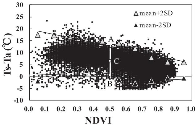
Fig. 3. The trapezoidal shape of Ts-Ta and NDVI to derive the iTVDI. The upper line indicates the dry edge, and the lower one indicates the wet edge. The iTVDI at point C is equal to BC/AB.
