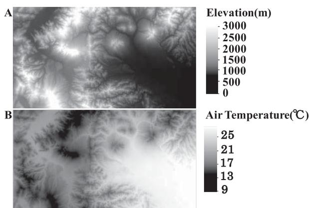
Fig. 2. The DEM of the study area (A) and the interpolated Ta map after a DEM calibration (B).
