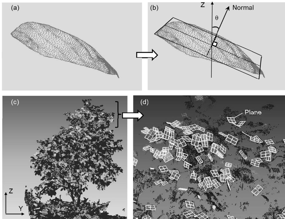
**Fig. 1.** Estimation of LIA from the high-resolution portable scanning lidar data. (a) An example of a set of points corresponding to a leaf. (b) A plane fitted to a point set of a leaf.  $\theta$  is the LIA, derived from the angle of the normal with respect to the zenith. (c) An example of planes fitted to each of 500 leaves within a 3-D point-cloud image. Shading effect by top light is added. (d) Close-up view of c, showing many planes fitted to leaves.
