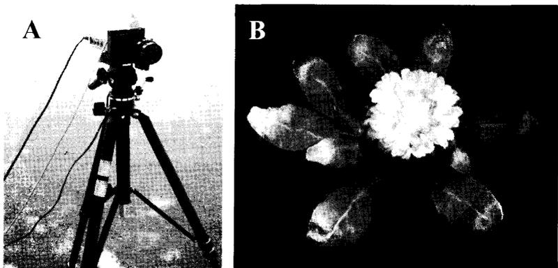
Figure 8. Passive 3-D color CCD camera (A) and 3-D texture mapping image (B) of flowering (pot marigold) plant calculated by a modified shape-from-focus (MSF) algorithm.
