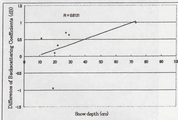
Fig. 3. Relationship between the difference of mean backscattering coefficients and snow depth.
