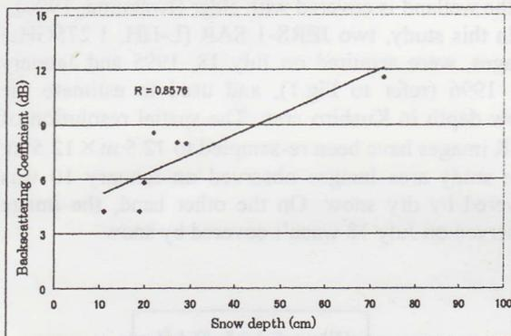
Fig. 2. Relationship between the mean backscattering coefficients and snow depth.
