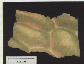
Fig. 10 Texture mapping image of pothos cells obtained by using a series of eight original color images that were illuminated in a checked pattern.
