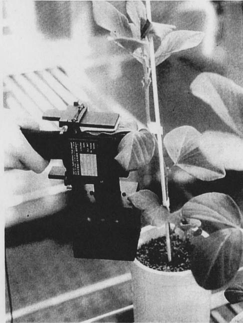
Fig. 4. Attachment with light source and integrating sphere for introducing light to spectroscopes via optical fibers
