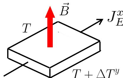
Transverse temperature gradient is produced in response to heat current
